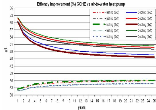
Figure 20: Heating and Cooling Efficiency Improvement GCHE vs. air-to-water Heat Pump for various borehole configurations
