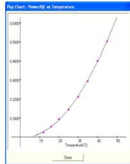
Figure 9: Electrical power consumed by the HP/Cooling Load vs entering temperature at the HP.
