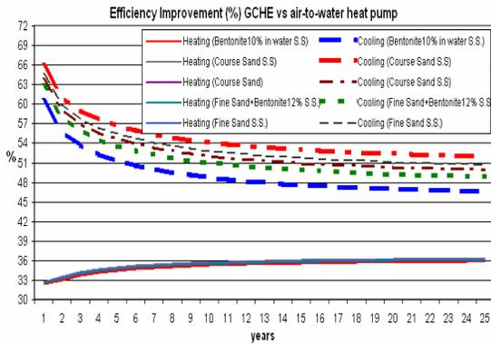
Figure 17: Heating and Cooling Efficiency Improvement GCHE vs. air-to-water Heat Pump for various Grouting Materials
