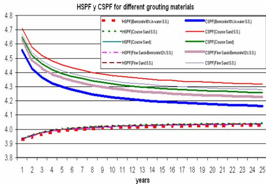
Figure 13: HSPF and CSPF for different grouting materials in a rectangular configuration (3x2)
