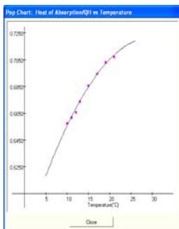
Figure 10: Heating capacity of the HP/Heating Load vs entering water temperature at the HP.
