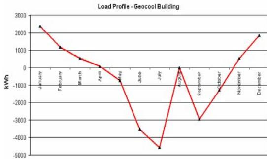
Figure1: Load Profile Geocool Building
