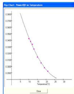
Figure 11: Electrical power consumed by the HP/Heating Load vs entering temperature at the HP.
