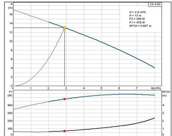
Figure 12: H-Q Curve for Grundfos CH 4-20 pump.
