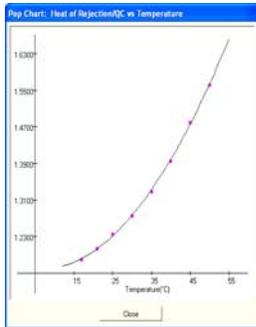
Figure 8: Cooling capacity of the HP/Cooling Load vs entering water temperature at the HP.
