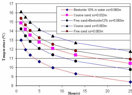
Figure 2: Modelling results for five different vertical borehole configurations in heating conditions.
