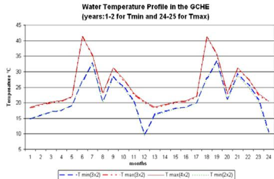
Figure 6: Maximum and minimum temperature profile of the water in the GCHE for some borehole configurations.
