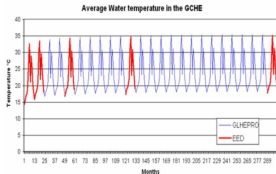
Figure 4: Average temperature profile of the water in the GCHE
