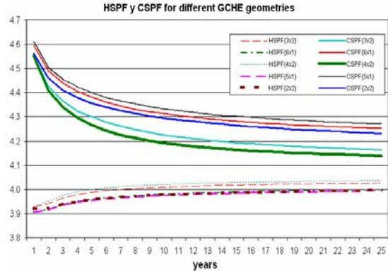
Figure 14: HSPF and CSPF for different borehole geometries
