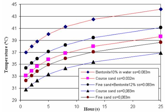
Figure3: Modelling results for five different vertical borehole configurations in cooling conditions.
