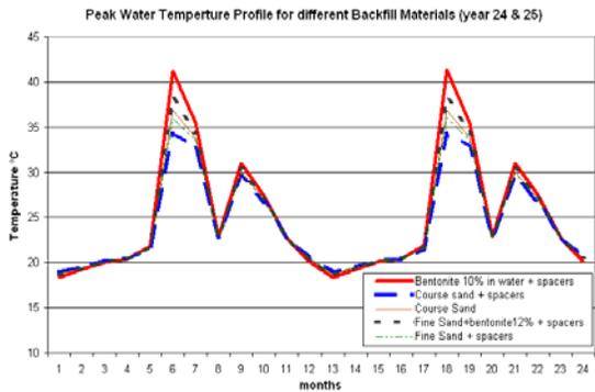
Figure 5: Peak temperature profile for the water in the GCHE for 5 kinds of backfill materials.
