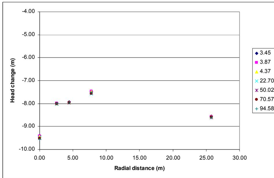
Figure 3. Change in piezometric head in the different observation wells, for different times (hours, see legend) during the experiment.
