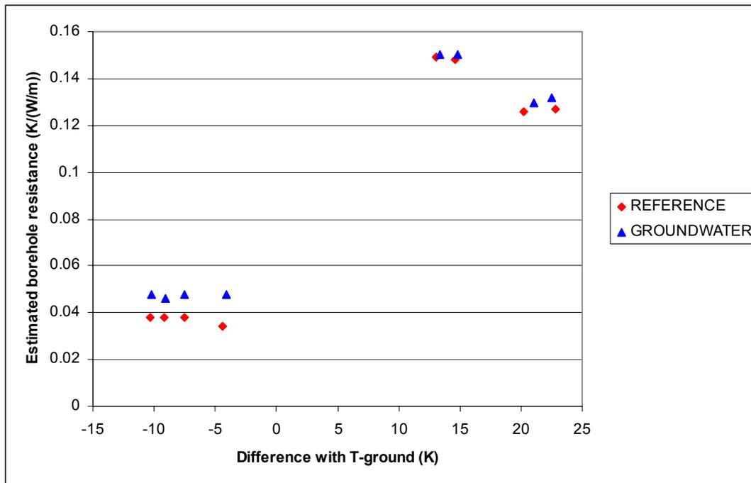
Figure 6: Calibrated borehole resistance values for 10-hour periods of the heat extraction and heat injection pulses plotted against the difference in average period temperature and undisturbed ground temperature.
