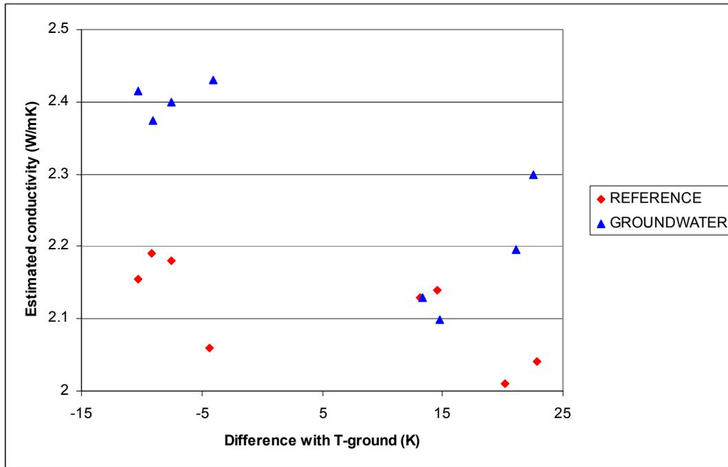
Figure 5: Calibrated conductivities for 10-hour periods of the heat extraction and heat injection pulses plotted against the difference in average period temperature and undisturbed ground temperature.
