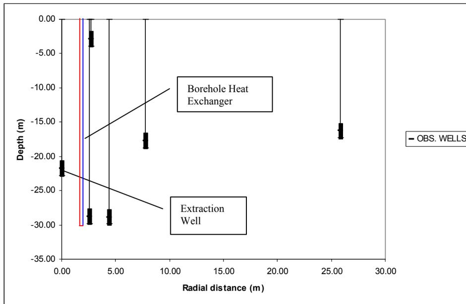
Figure 2: Observation well positions: filter depth and radial distance to extraction well.
