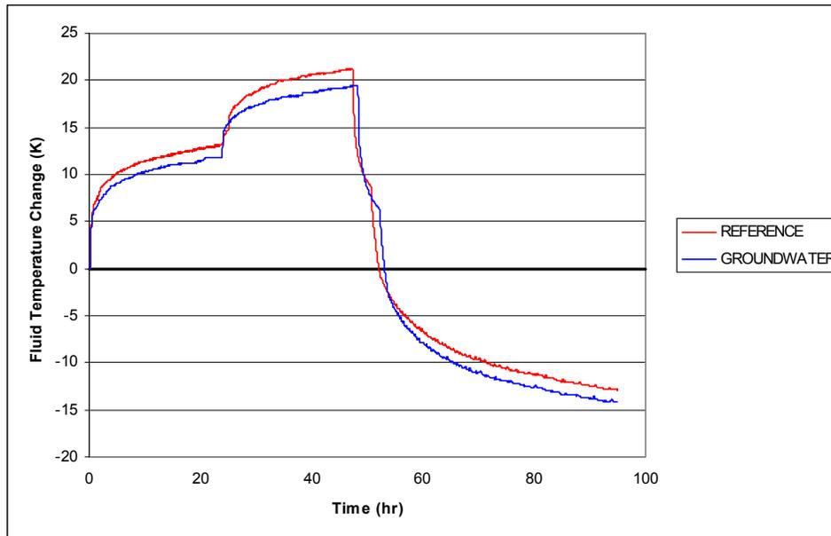
Figure 4: Temperature change of heat transfer fluid temperatures for the reference and groundwater extraction experiment.
