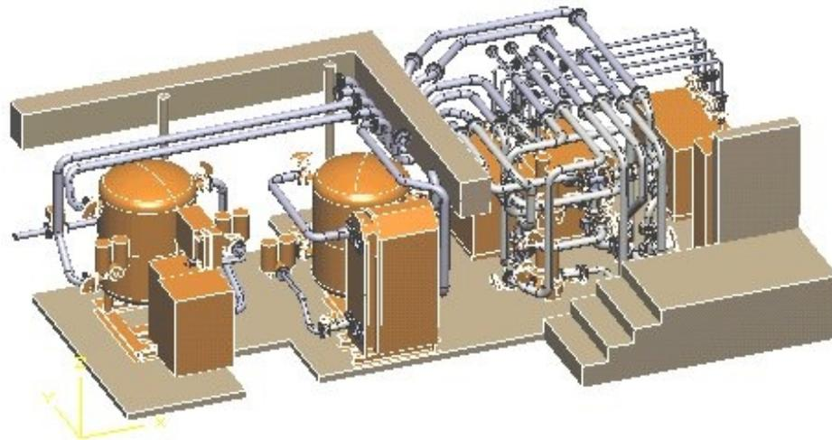
Figure 5 3D CAD drawing of heat pump energy plant design
