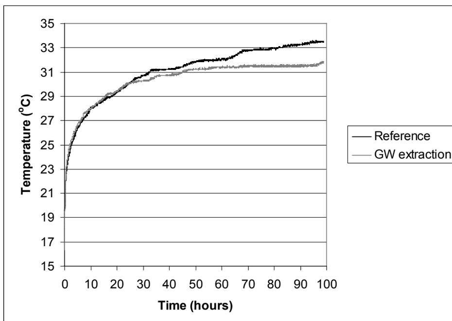
When we construct sensitivity graphs (figure 10) it is clear that the conductivity values estimated from the data of the reference experiment stabilise to values around 2.3 W/mK. For the experiment with groundwater extraction the estimated conductivity increase when more data is added.
