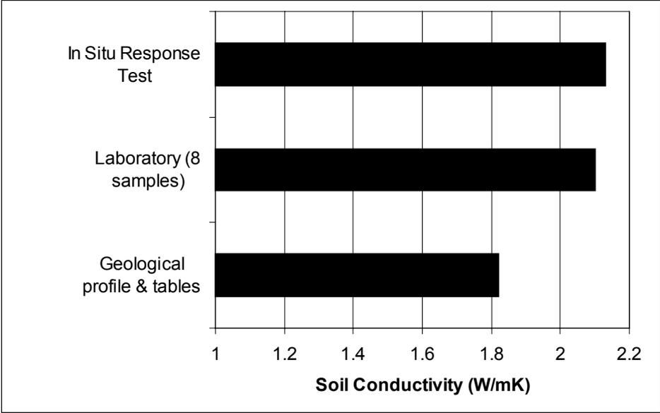
The second validation is based on ten tests that have been performed at the same site (located at the Groenholland offices in Amsterdam). The average thermal conductivity found is 2.16 W/mK, with individual measurements ranging between 2.08 and 2.29 W/mK. Interesting is that there appears to be a positive linear relationship between thermal conductivity and (positive) watts applied, which could be an indication of increasing convection in the borehole during heat-injection.
