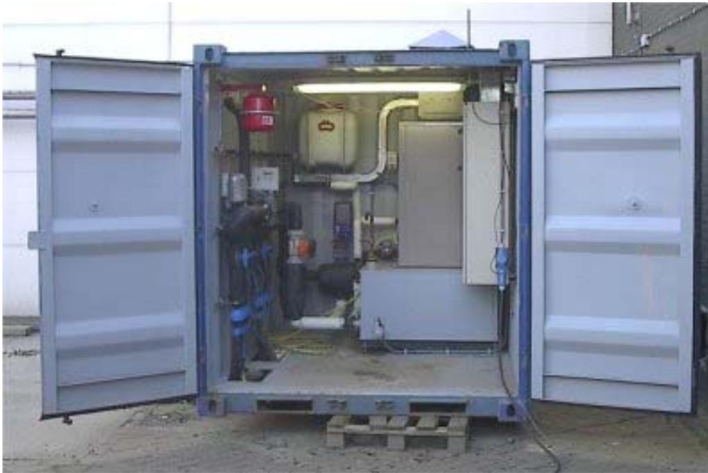
During the experiment temperatures, flow rate and pressure are logged at regular intervals (usually 240 or 480 seconds). The pressure sensor is used to switch off the system automatically when a calamity occurs (when the pressure drops below a selected value). The whole system is controlled by an on-board computer and incorporates a GSM modem for remote system management and data logging.
