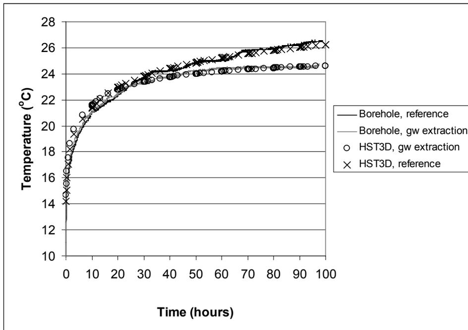
Subsequently we used this model to calculate the response of a groundloop heatexchanger with different groundwater flow regimes (figure 12). When these temperature series are used to estimate the apparent thermal conductivity (figure 13) of the ground we can observe that the estimated ground thermal conductivity increases dramatically with groundwater flowrates. A significant effect is already noticeable at small flowrates (Darcy flow < 3.5 m/yr, 6% higher conductivity estimate).
