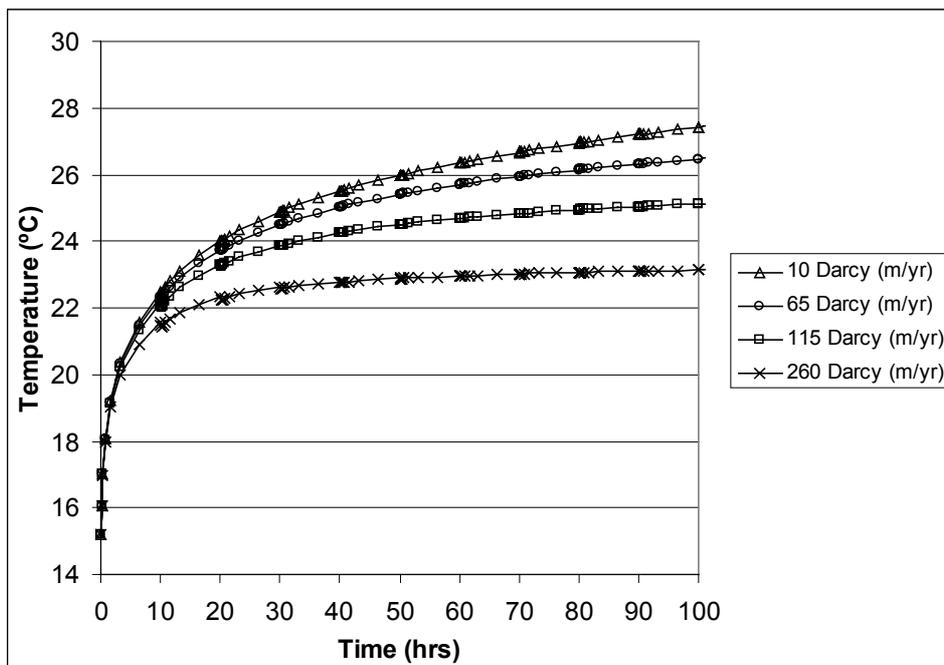
**Figure 13.** Estimated thermal conductivity with no groundwater flow and estimated apparent ground thermal conductivity simulated temperature response at different groundwater flowrates.
