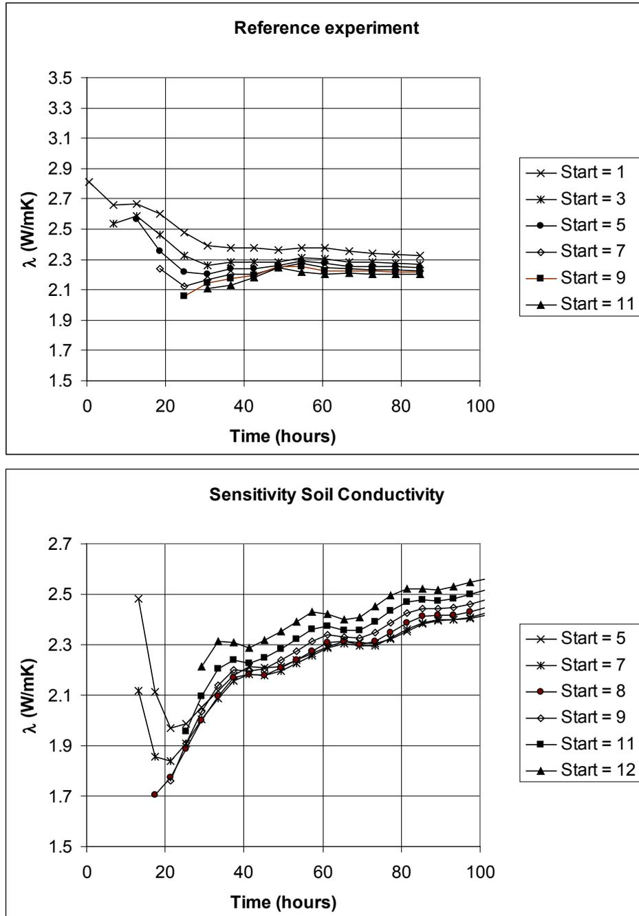
**Figure 11.** Correspondence between observed and simulated thermal response (HST3D) for the reference experiment and experiment with groundwater extraction.
